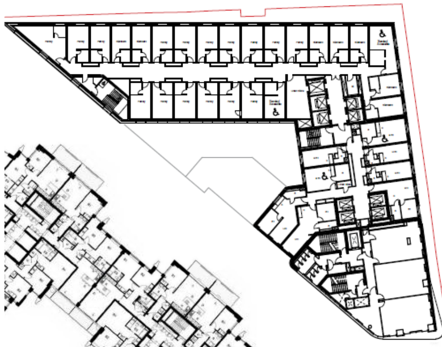
Approved and as proposed 5 th floor showing hotel and serviced apartments and school to southern tip of building.
